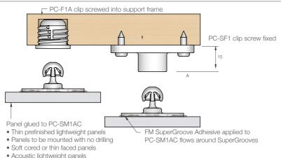
The Fastmount® multi-award winning system has revolutionized the mounting of panels. Panels can easily be removed and refitted in any sequence time after time. For further information or technical support contact: info@fastmount.com
